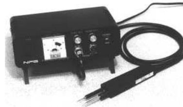
Hot probe for silicon ingot
